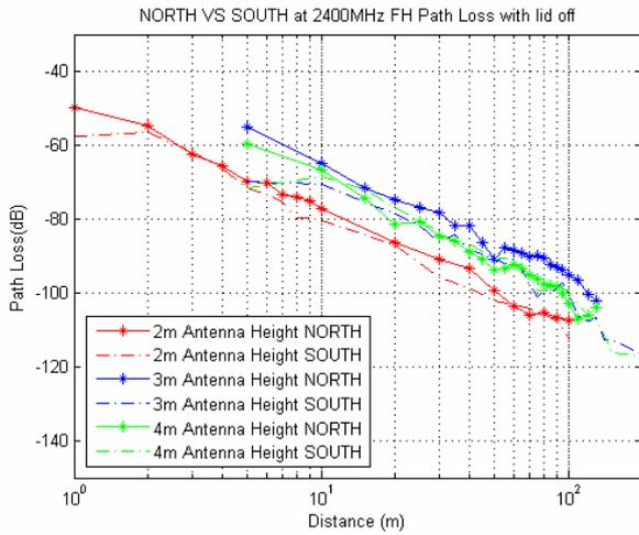
Fig.8. 2400MHz Direction Analysis lid off
