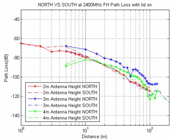
Fig.7 2400MHz Direction Analysis lid on
