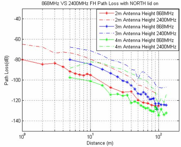
Fig.5 868MHz vs 2400MHz lid on
