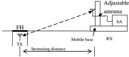
Fig.4 Field Measurement setup (2D)
