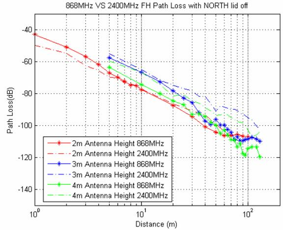
Fig.6 868MHz vs 2400MHz lid off
